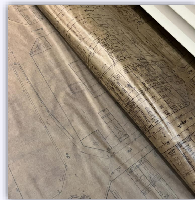
Deformations resulting from dimensional changes
