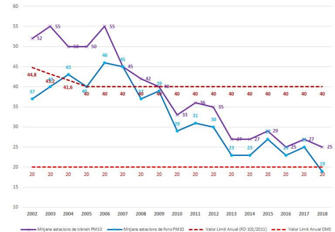
Evolution of the annual average for immissions of PM 10 recorded by the XVPCA stations in Barcelona [µg/m 3 ]
